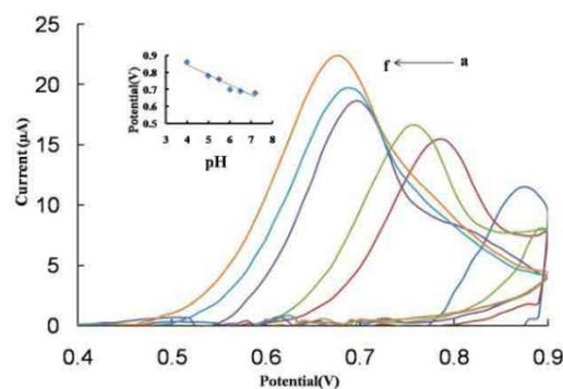
**Fig. 3.** Background subtracted cyclic voltammograms of 0.1 mM AMT at the NC-CILE; pH from a to f: 4.0, 5.0, 5.5, 6.0, 6.5, 7.2 at  $50 \text{ mVs}^{-1}$ , accumulation time 240 s and accumulation potential 0 V. Inset: plot of oxidation peak potential vs. pH.
