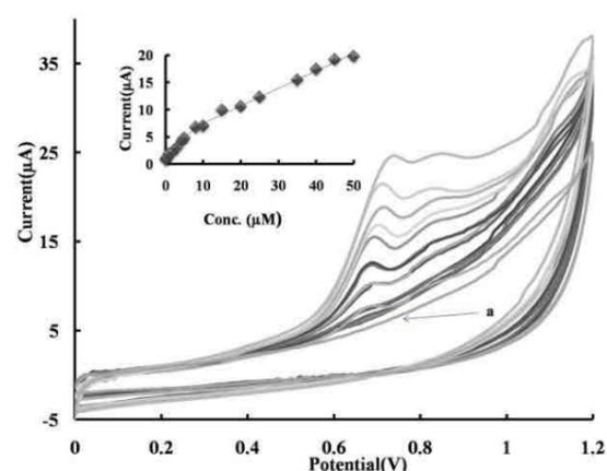
**Fig. 6.** Cyclic voltammograms of NC-CILE in 0.07 M PBS, pH 7.2 in the presence and (a) in the absence of different concentrations of AMT measured, accumulation time 240s and accumulation potential 0 V. Inset shows the calibration curve of peak current vs. AMT concentration.
