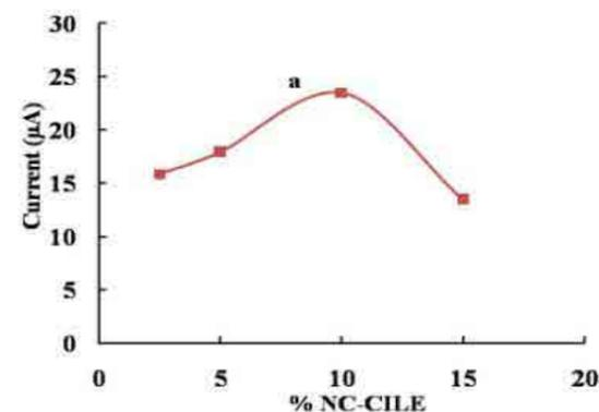
**Fig. 4.** The influence of % NC-CILE on the anodic peak current of 0.1 mM AMT in PBS 0.07 M (pH 7.2) at a scan rate of  $50 \text{ mVs}^{-1}$ .
