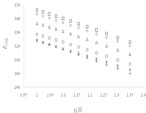
**Fig. 1.** Experimental *emf* values versus  $p_c H$  in ionic strength of 0.10 (+), 0.50 (\*), 1.00 (O), 1.50 ( $\Delta$ ), 2.00 ( $\diamond$ ) and 3.00 ( $\square$ ) mol  $\text{dm}^{-3}$   $\text{NaClO}_4$
